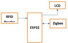
The Zigbee transceiver module provides wireless communication between the classroom ESP32 unit and the staff room monitoring system. This transmits processed lecturer tracking data to the central monitoring unit in the staff room, where it is integrated to the web application. Zigbee is chosen because of its low power consumption, reliability and mesh networking capability, which makes it ideal for multi classroom setups, especially across large campuses.
