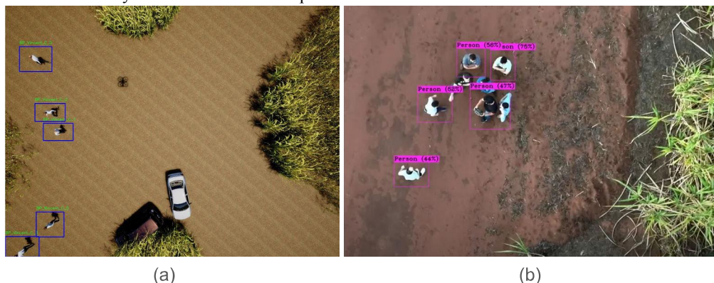
FIGURE 8. (a) Person detection ground truth in simulated scenario (b) Person detection in real-world image with fine-tuned YOLO model.
