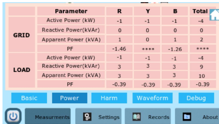
Figure 6.3: Power measurement screen showing active and reactive power data.
