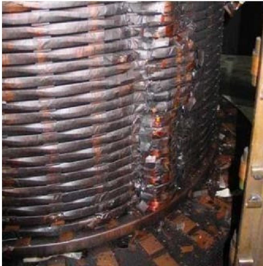
Fig. 2.2 Radial buckling of inner winding [4].
