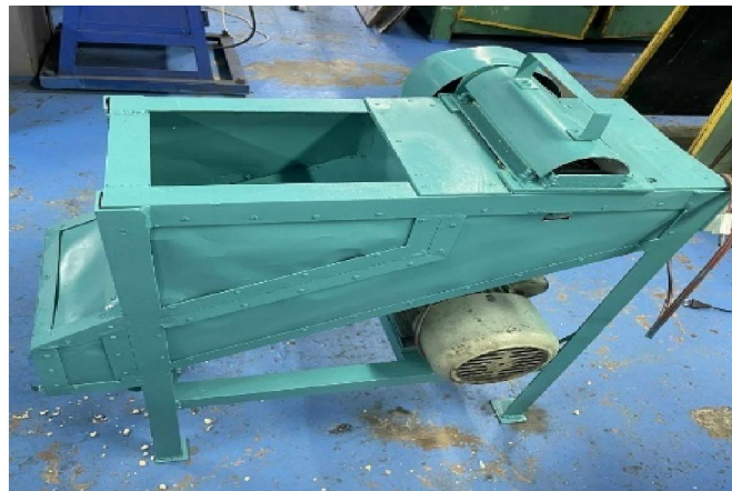
Figure 3. The Prototype Corn Manual Corn Sheller
