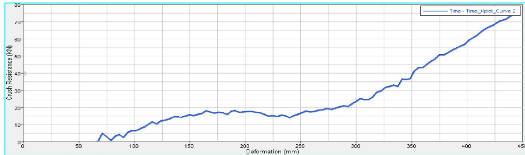
Fig. Crush resistance vs Deformation graph of S shaped steel intrusion beam.
