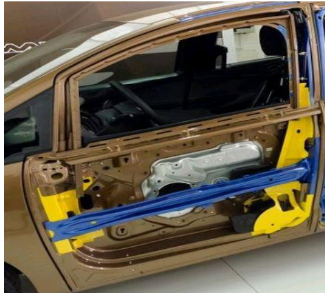
Fig.1.1 Intrusion beam inserted in actual side car door model.
