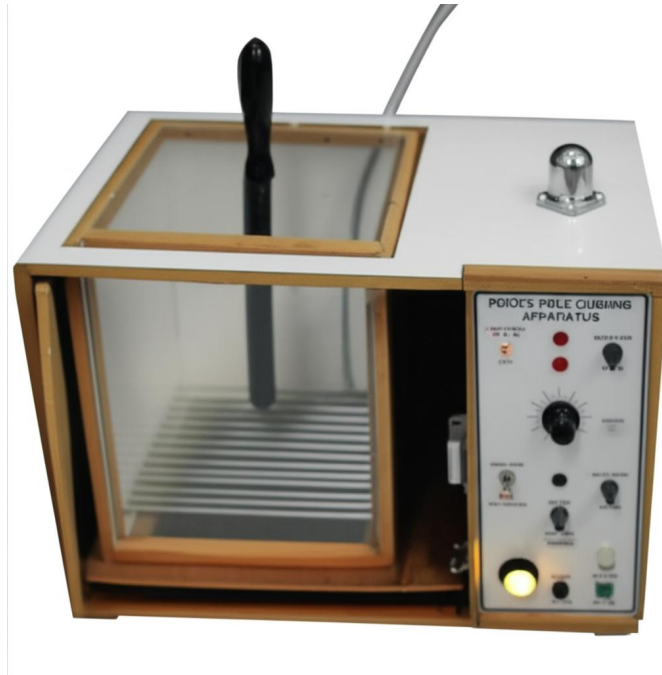
Figure 04: COOK'S POLE CLIMBING APPARATUS
