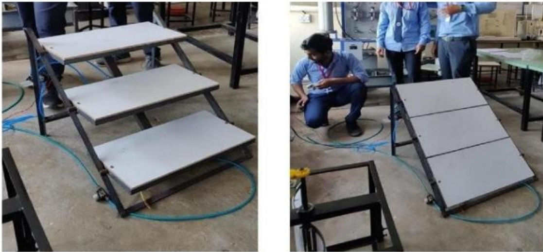
Figure 2. Actual Working Model of Convertible Staircase to Ramp Project.
