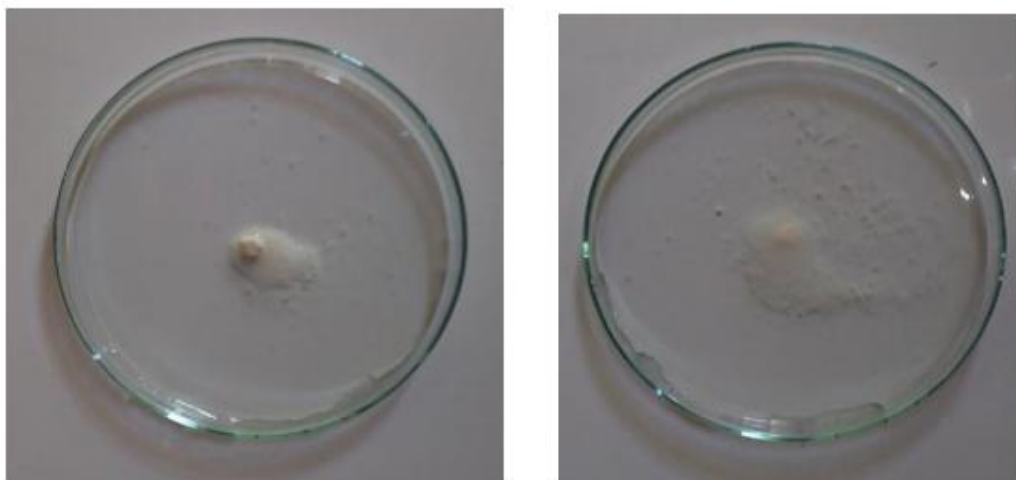
Fig 4: Dispersion time of Metoclopramide HCl tablets prepared by Direct Compression method
