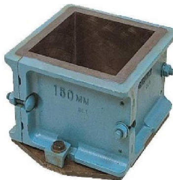
Fig. 3: Moulds/ Cubes for Testing
