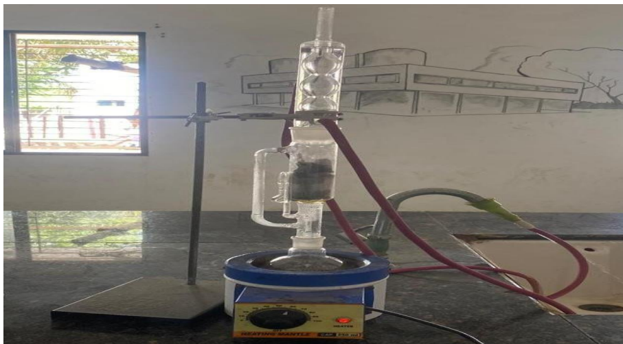
Fig. Schematic of a Soxhlet extraction apparatus indicating the vapor and liquid extractant paths. The sample under extraction is cushioned by loosely packed ceramic fibers.
