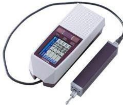
Figure 4. Tally Surf Surface Roughness Tester
