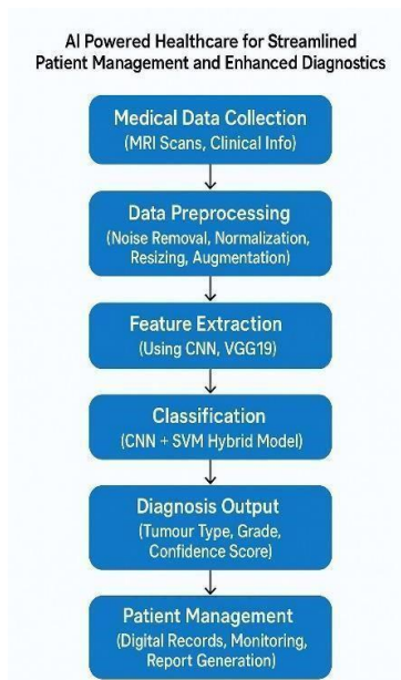
Fig. 1. Workflow of AI Powered HealthCare For Streamlined Patient Management and Enhanced Diagnostics For Brain Tumour
