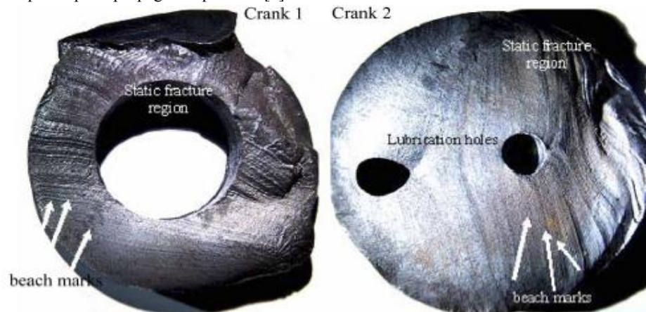
Fig .5.2.Failed crankshaft and their fracture surfaces at sharp fillet region.
