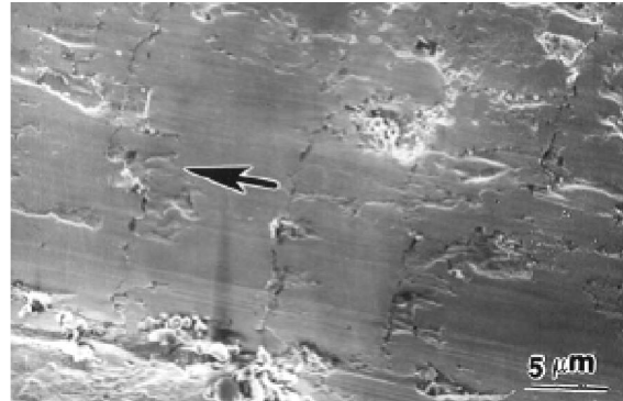
Fig. 6.12 SEM shows pitting, spalling and surface cracking at web radius
