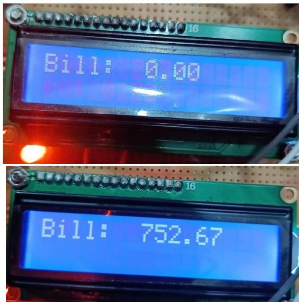
Fig 3. Results of the water flows and bill amount on LCD screen
