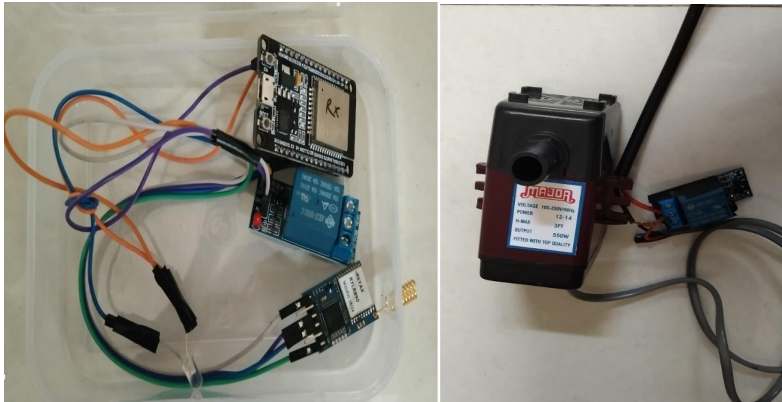
Fig.3. Transmitter and Receiver of Smart water pump controller
