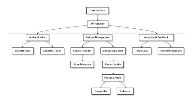
The Authentication Module ensures secure access to the system. It consists of two key processes: user validation and token generation. The system verifies credentials to confirm user authenticity and then generates a secure token to maintain an active session during usage.
