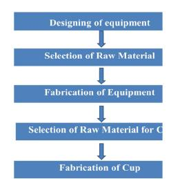
The design and development of bio cups from corn husk begins with sourcing the husks, a Common agricultural waste product. The husks are cleaned thoroughly to remove dirt, dust, and any contaminants before being dried to reduce moisture content. The husk fibers are then mixed with natural binders like starch or cellulose to improve the material's moldability and strength. This mixture is molded into cup shapes using compression or injection molding techniques,
