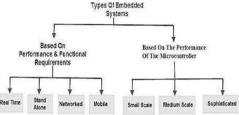
Embedded systems are primarily classified into different types based on complexity of hardware & software and microcontroller (8 or 16 or 32-bit). Thus, based on the performance of the microcontroller, embedded systems are classified into three types such as:
