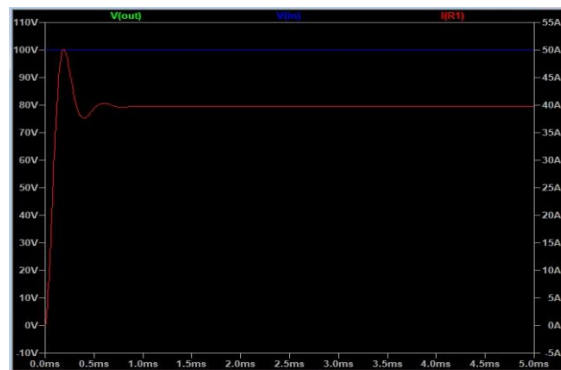
Fig 10: Simulation Result of Charging stage Buck converter
