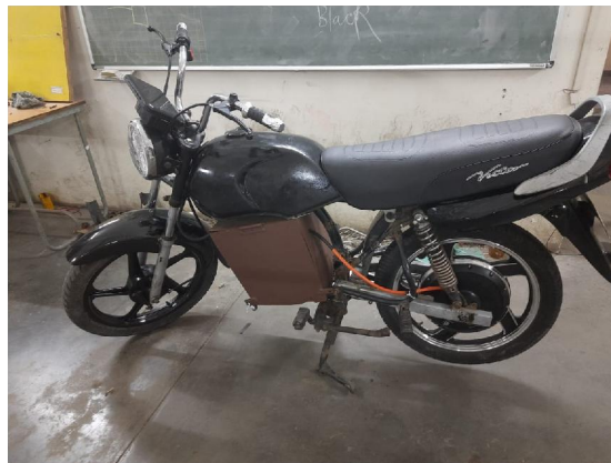
Fig 13: Complete retrofit motorbike
