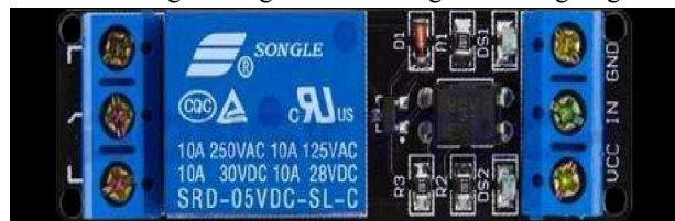
Fig 10: 1 Channel Relay module with Optocoupler
