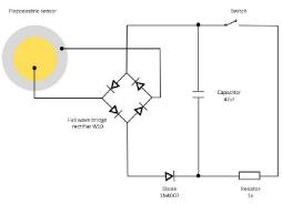
The energy conversion process begins with piezoelectric transducers embedded in tiles, capturing mechanical force from footfalls. The resulting alternating current (AC) is converted into direct current (DC) through a full-wave bridge rectifier. The rectified DC is then filtered and stored in capacitors or batteries, making it suitable for low-power applications like streetlights and digital signboards.
