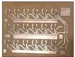
To optimize energy output, the piezoelectric transducers are arranged in different configurations—series, parallel, and series-parallel. A series connection generates higher voltage but lower current, whereas a parallel connection increases current but reduces voltage. To strike a balance, a series-parallel configuration is implemented, ensuring an optimal combination of both voltage and current.
