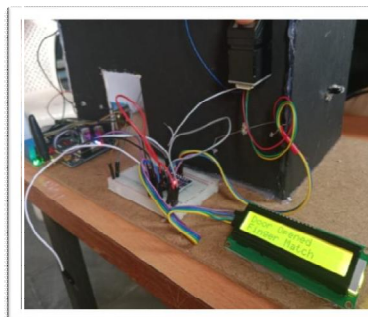
Figure 3: When door is opened after fingerprint verification and buzzer activated when detected suspicious activity.
