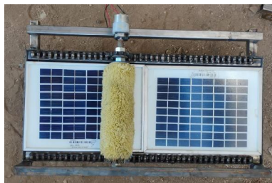
Figure 1. Automated Solar Panel Cleaning Mechanism Using Rotary Brush System
