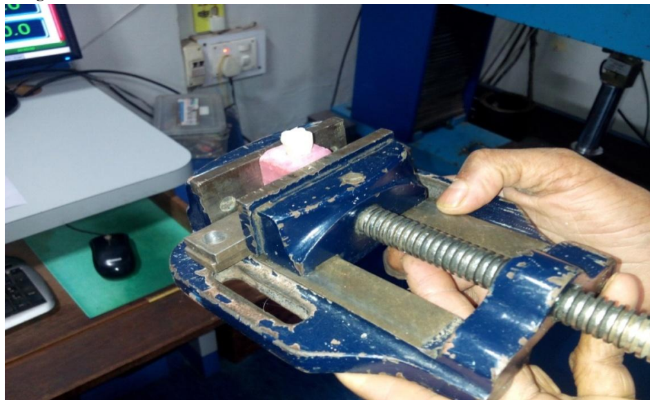
Figure 4.2: Tooth holding fixture
