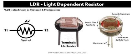
Light Sensing: The primary function of the LDR is to detect changes in light intensity. LDRs are passive components whose electrical resistance varies based on the amount of light falling on them. When exposed to light, the resistance of the LDR decreases, and when in darkness, the resistance increases.
