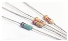
A resistor is a passive two-terminal electrical component that implements electrical resistance as a circuit element. Resistors act to reduce current flow, and, at the same time, act to lower voltage levels within circuits. In electronic circuits, resistors are used to limit current flow, to adjust signal levels, bias active elements. And terminate transmission lines among other uses.
