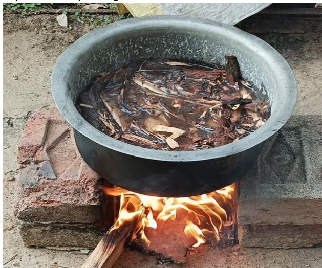
Fig. 3.3 Preparation of Cypress Tree Extract Admixture
