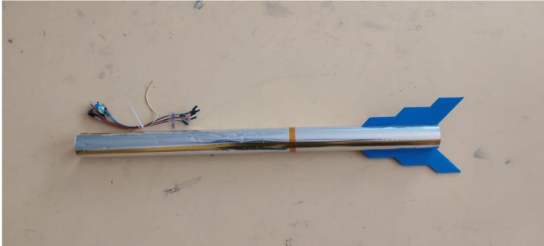
Airframe of Rocket made by PVC Material
