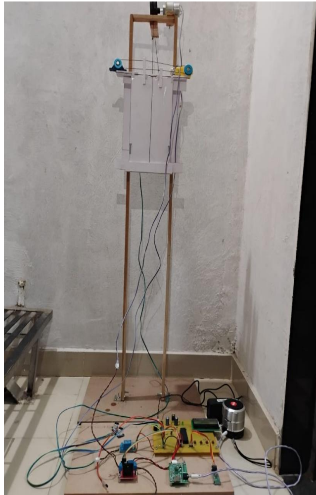
Fig :voice operated lift control system with safety
