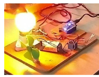
Breathing Input3: Bulb ON/OFF (Exhalation)
