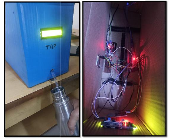
The setup part runs once when the system starts. It initializes the RFID reader, the LCD display and other components. It also loads the information about the users into memory (from EEPROM) and displays "System Ready" on the LCD. In the loop (which runs continuously), the system waits for the RFID card to be scanned: o If a card is scanned:
