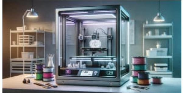
The 3D printing process turns an object into many, tiny little slices, then builds it from the bottom-up, slice by slice. The layers then build up to form a solid object. The process of building objects in this way is also referred to as Additive Manufacturing.Not all 3D printers use the same technology. There are several ways to print and all those available are additive, differing mainly in the way layers are built to create the final object.
