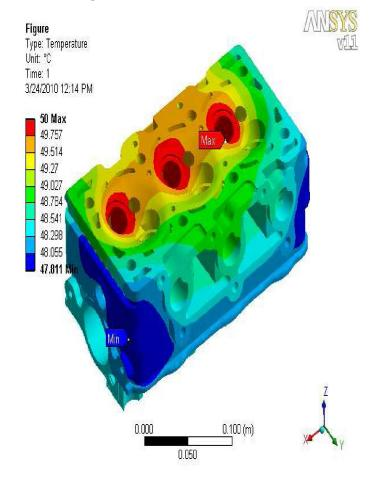
CASE I: Coolant flow rate of 80 GPM
