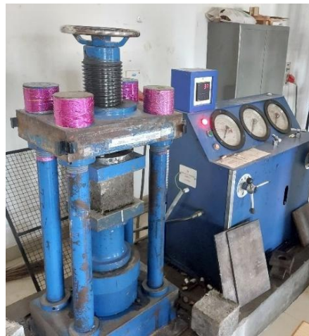
Figure 3 Testing of concrete
