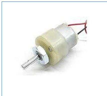
DC Motor – 60RPM – 12Volts geared motors are generally a simple DC motor with a gearbox attached to it. This can be used in all-terrain robots and variety of robotic applications. These motors have a 3 mm threaded drill hole in the middle of the shaft thus making it simple to connect it to the wheels or any other mechanical assembly. 60 RPM 12V DC geared motors widely used for robotics applications.
