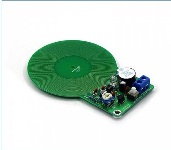
we can use this Metal detector non-contact metal induction detection module as a metal detector. When it approaches any metal, it makes a sound.
