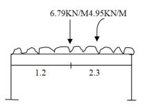
MAXIMUM LOAD MAXIMUM INTENSITY TOTAL LOAD = UDL +WALL LOAD 4.9+ 9KN = 13.95 KN/M LOAD + WALL LOAD
