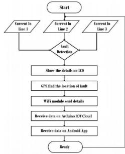
At first, we power up or start the project and it is going to read the three- phase line .if our program detects the fault in line then it sends the data to user and if not occurred any fault, then keep sensing the fault. Every time it checks the conditionand continuously run in a cycle or loop.
