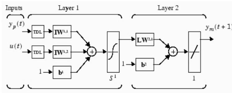
Figure 8. The internal structure of neural network model
