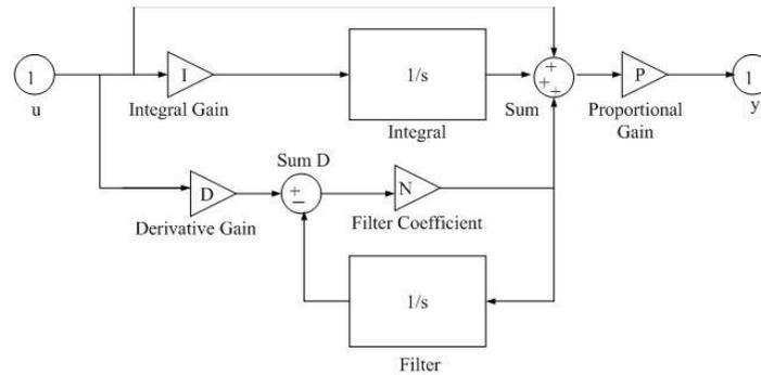
Figure 6. PID controller
