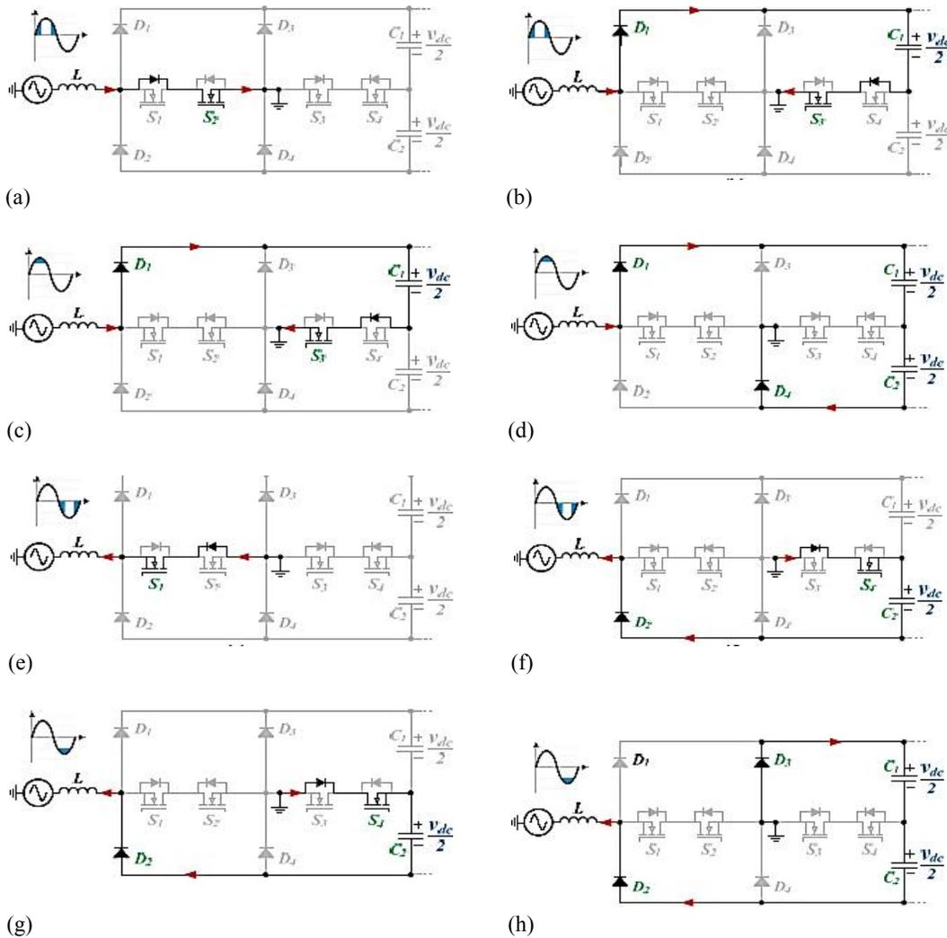
Figure 2. The step-by-step operation of the proposed five-level active rectifier (a) stage output 0 V to  $V_{dc}/2$ , (b) stage output 0 V to  $+V_{dc}/2$ , (c) stage output  $+V_{dc}/2$  to  $+V_{dc}$ , (d) stage output  $+V_{dc}/2$  to  $+V_{dc}$ , (e) stage output 0 V to  $-V_{dc}/2$ , (f) stage output 0 V to  $-V_{dc}/2$ , (g) stage output  $-V_{dc}/2$  to  $-V_{dc}$ , and (h) stage output  $-V_{dc}/2$  to  $-V_{dc}$
