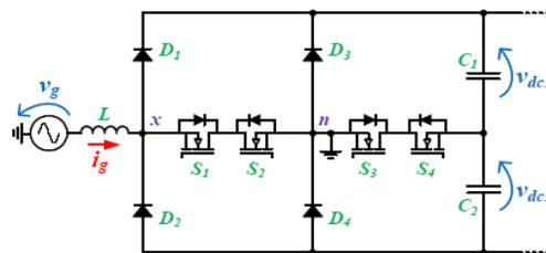
Figure 1. Five-level active rectifiers for EV battery chargers
