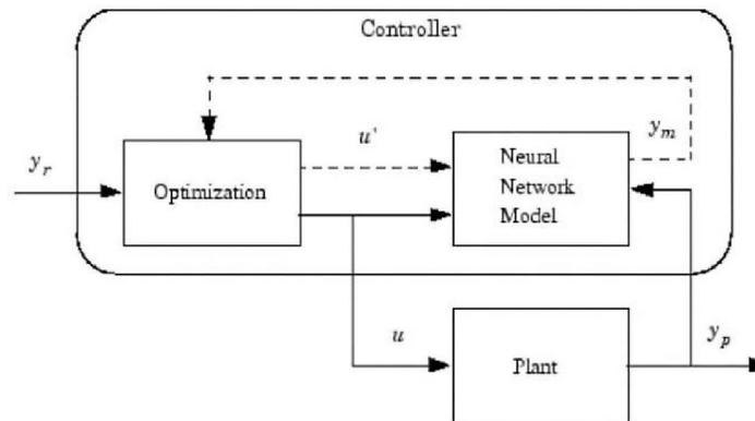
Figure 9. Control process in the network model
