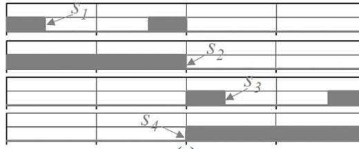
Figure 3. MOSFET switch pulse pattern
