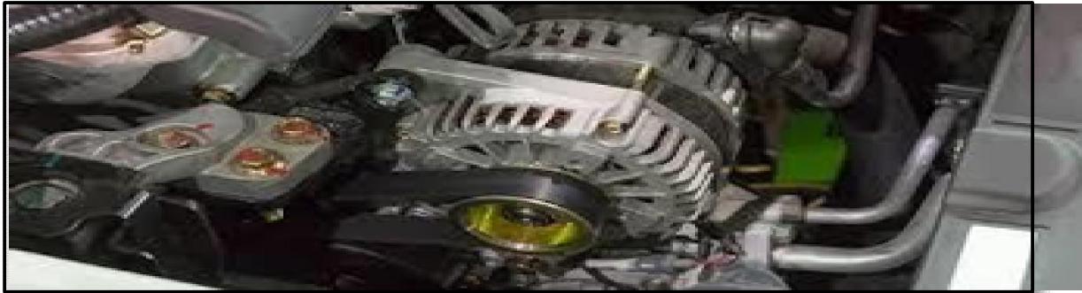
Figno.4 Charging Unit
