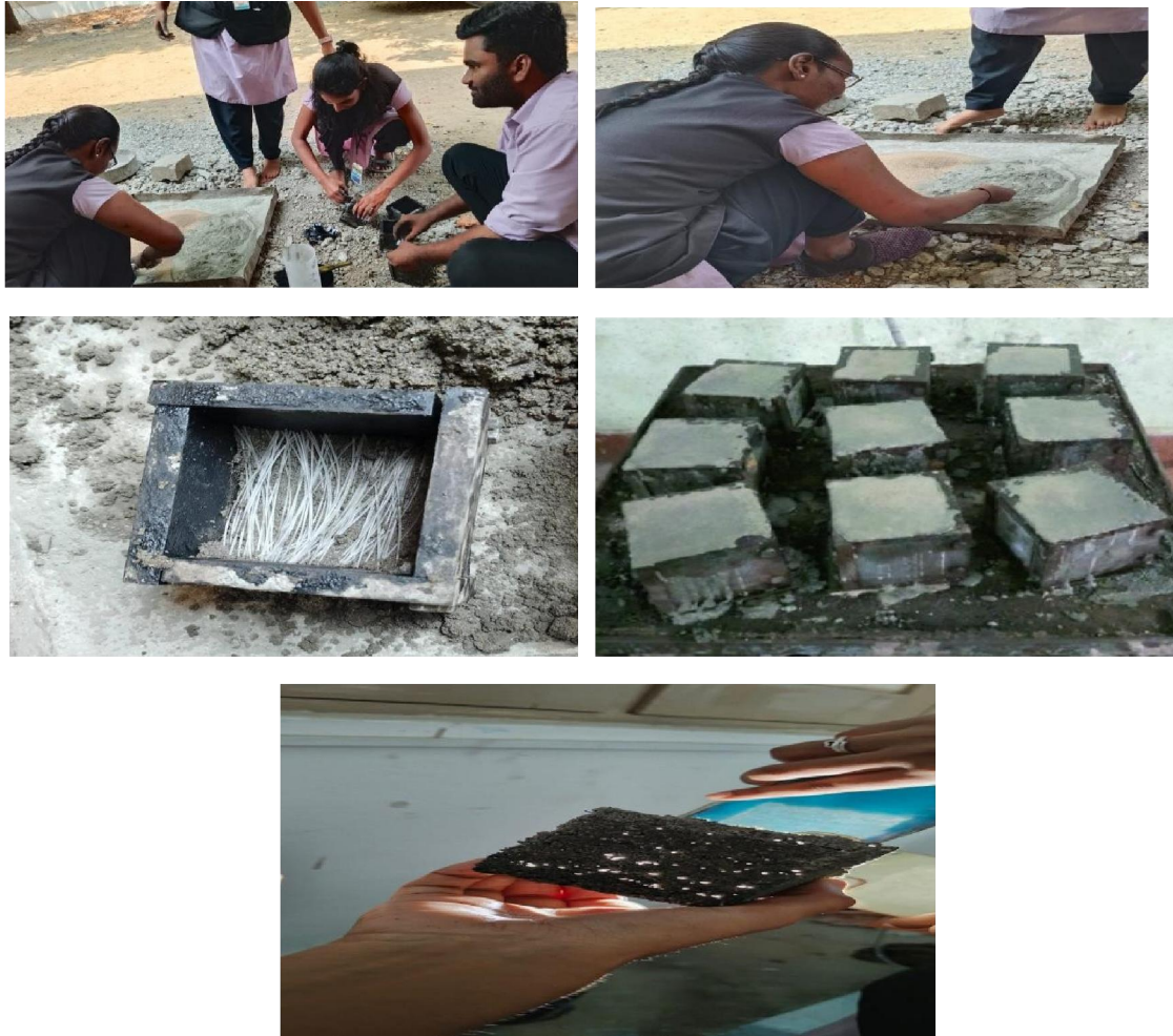
Fig. 1 Casting Of Moulds
