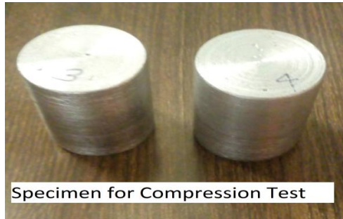
Fig 5. Test specimen for compression test
