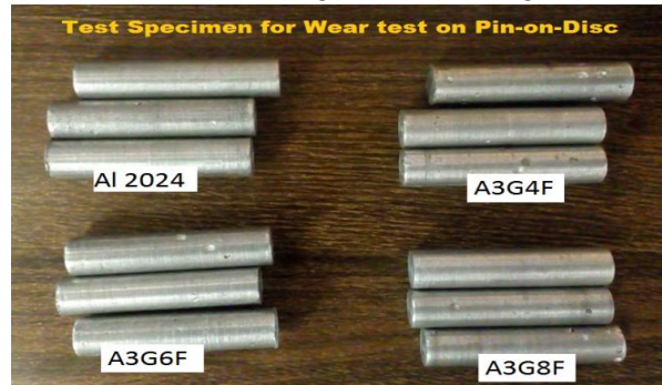
Fig 6. Test specimen prepared for wear test (before test)
