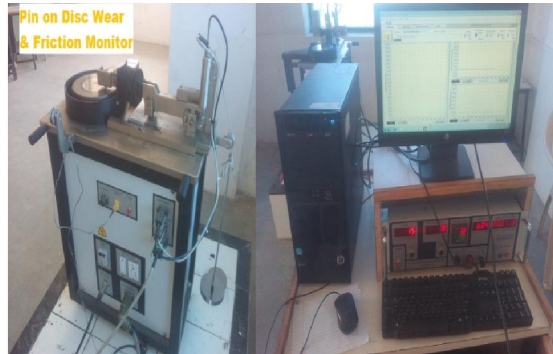
Fig 13. Wear and Friction Monitor (Pin-on-Disc)
