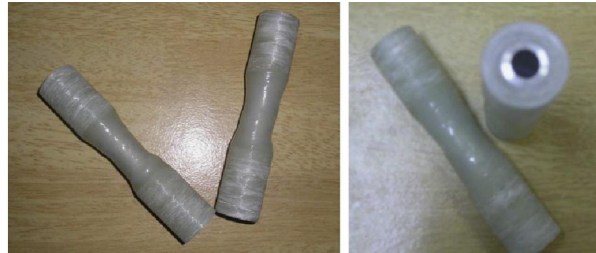
Fig.4. Sample of hybrid aluminum/composite fatigue specimens used.
