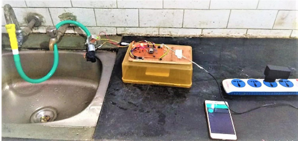
Figure 5: Working Model of IoT based Electric Valve
