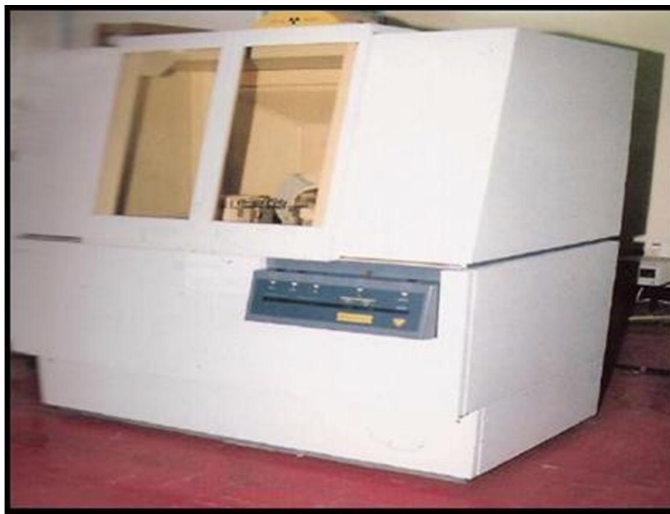
Fig.3.5 Philips X-pert multipurpose x-ray diffractometer
