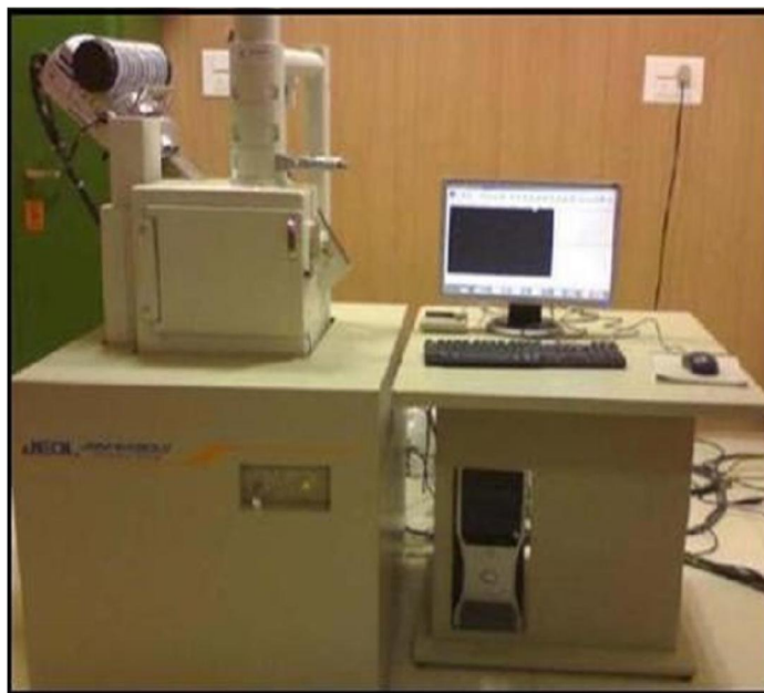
Fig. 3.4 Scanning Electron Microscopy (JEOL JSM-6480LV)
