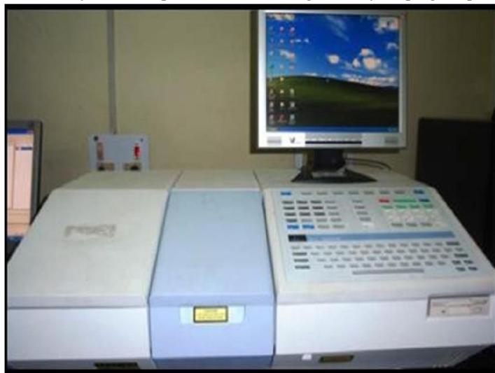
Fig.3.6 Perkin-Elmer Spectrum RXI, (FTIR) Spectrometer
