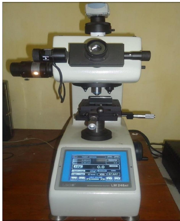
Fig. 3.1- Leco, LM 248AT Micro indentation Hardness Tester
