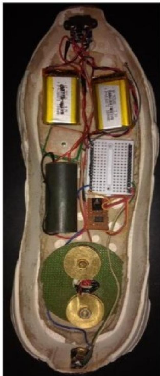
Fig.7: Shoe (Node MCU, Shockwave Generator, Buzzer, Battery).
