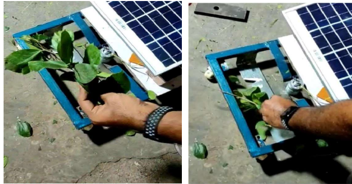
Fig. 2. Fixation of Blade to Solar grass Cutter
