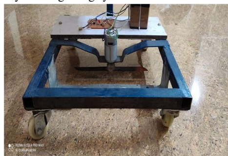
Fig. 6. Wheels connected with DC motor DOI: 10.48175/IJARSCT-13662
