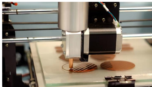
Figure 3 Popular 3D food machines work similarly to FDM 3D printers[3]
