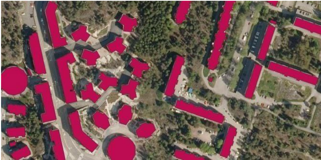
Figure 3: An example of building detection from the ATMU UNet model.
