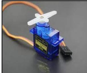
Figure 6: SG90 Servo Motor
