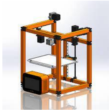
Fig. 2: Cartesian FDM 3D printers
